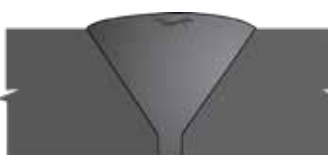
20 Crater Crack (crown stop-start area) MT/PT, UT
