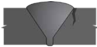
10 Toe Crack in Single Vee MT/PT, UT
