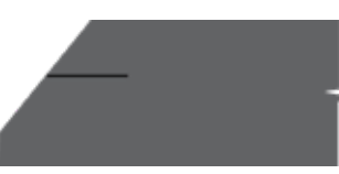
51 Lamination in Weld Prep MT/PT, UT
