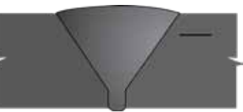
50 Lamination in Single Vee (base metal) UT
