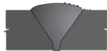
90 Weld Splatter on Single Vee, VT, RT
