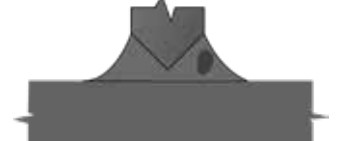
38 Slag Inclusion in Fillet (root area) UT, RT
