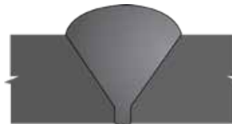
74 Excess Crown in Single Vee, VT
