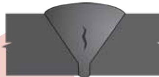
15 Centerline Crack, Single Vee (sub-surface) UT, RT
