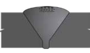
32 Porosity in Single Vee (surface breaking) VT, MT/PT
