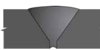
70 Root Concavity in Single Vee VT, RT
