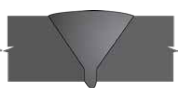
71 Excess Root Penetration in Single Vee VT, RT
