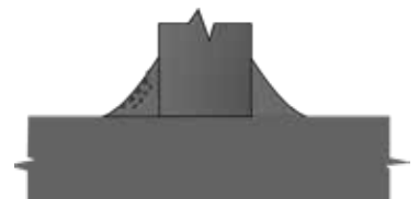
33 Porosity in Fillet (surface breaking) VT, MT/PT
