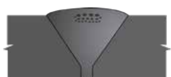
30 Porosity in Single Vee (sub-surface) UT, RT
